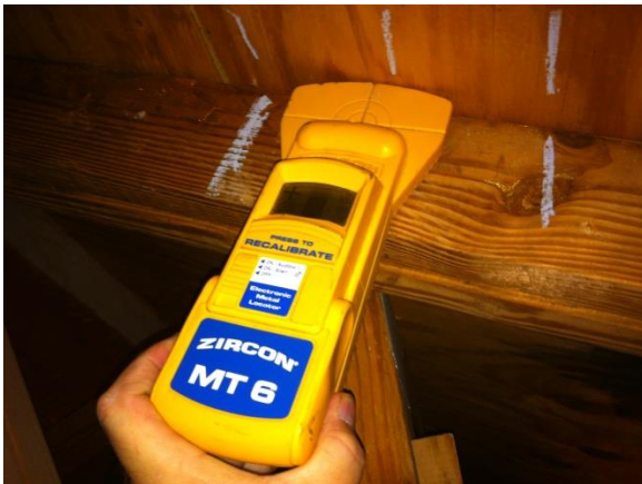
ZIRCON METAL DETECTOR TO IDENTIFY NAIL LOCATIONS.
