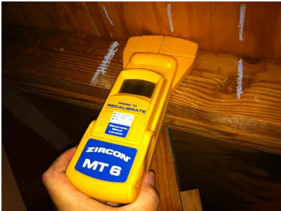
ZIRCON METAL DETECTOR TO IDENTIFY NAIL LOCATIONS.
