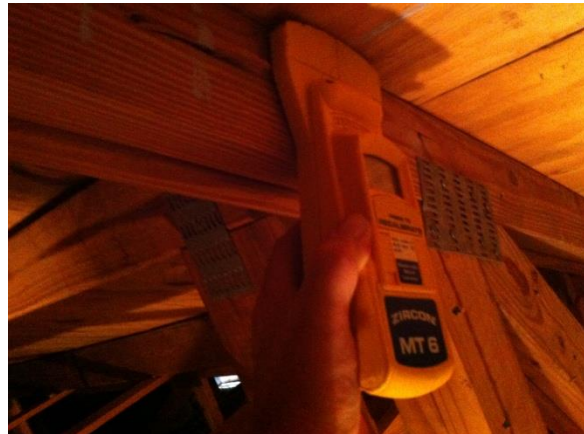
ZIRCON METAL DETECTOR TO IDENTIFY NAIL LOCATIONS.
