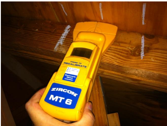
ZIRCON METAL DETECTOR TO IDENTIFY NAIL LOCATIONS.
